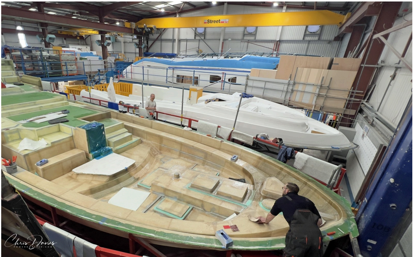
A hull under construction in the GRP facility. Photo: Chris Davies / Powerboatpix.com
